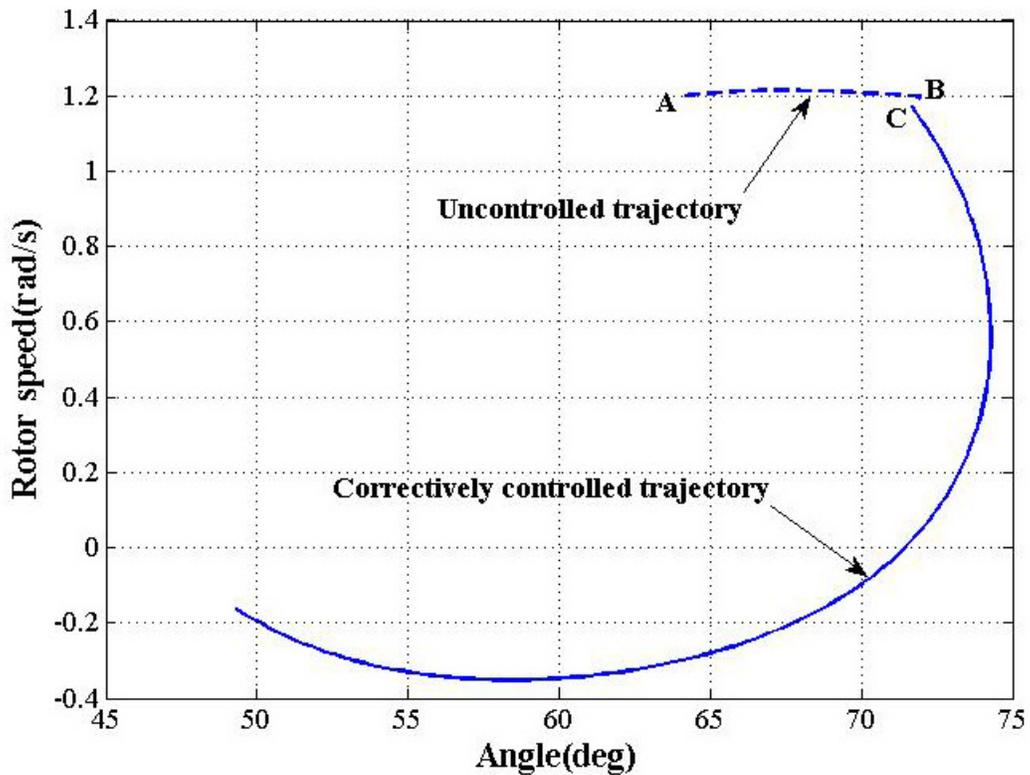
Figure 4.20 OMIB equivalent phase plane for case 1NE: Stabilized system.
