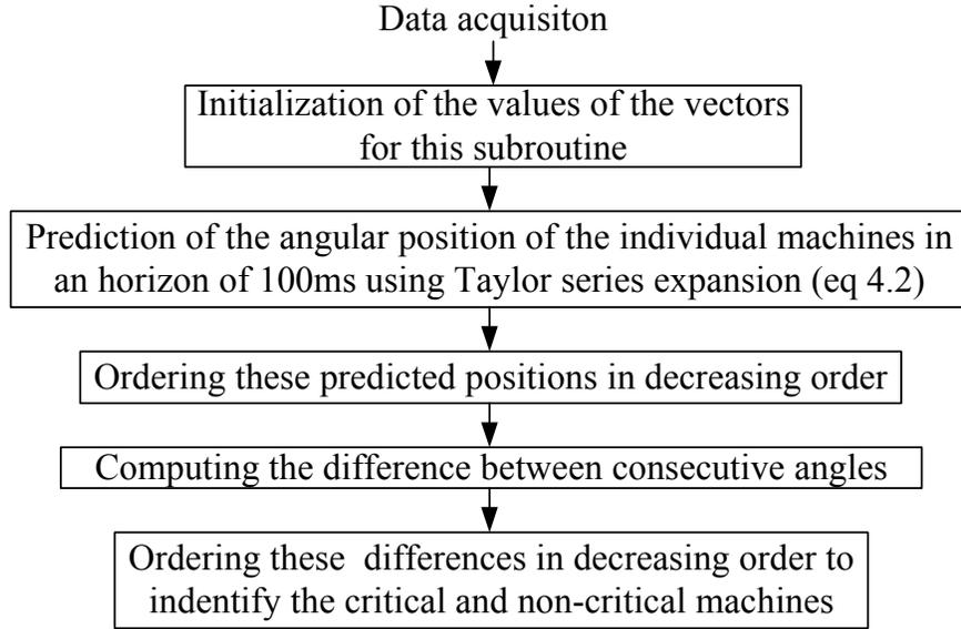
Figure 3.12 Flow diagram of the prediction step of individual machines' angles.
