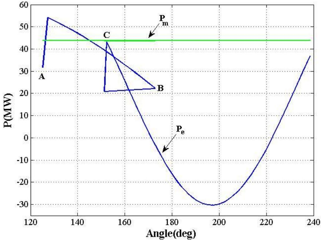
Figure 4.11 OMIB equivalent mechanical and electrical powers for case 2A.
