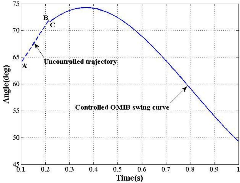
Figure 4.19 OMIB equivalent swing curve for the case 1NE: Stabilized system.
