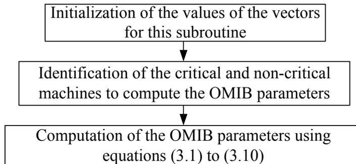
Figure 3.13 Flow diagram of the computation of the OMIB parameters.
