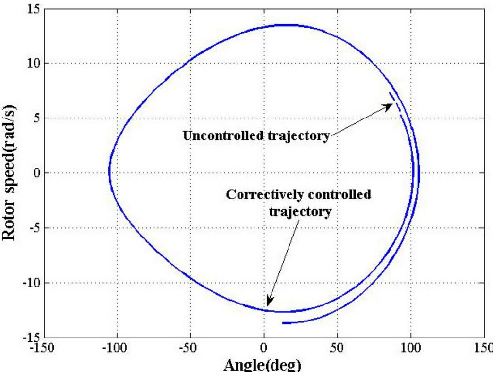
Figure 4.26 OMIB equivalent phase plane for case SIEQ: Stabilized system.
