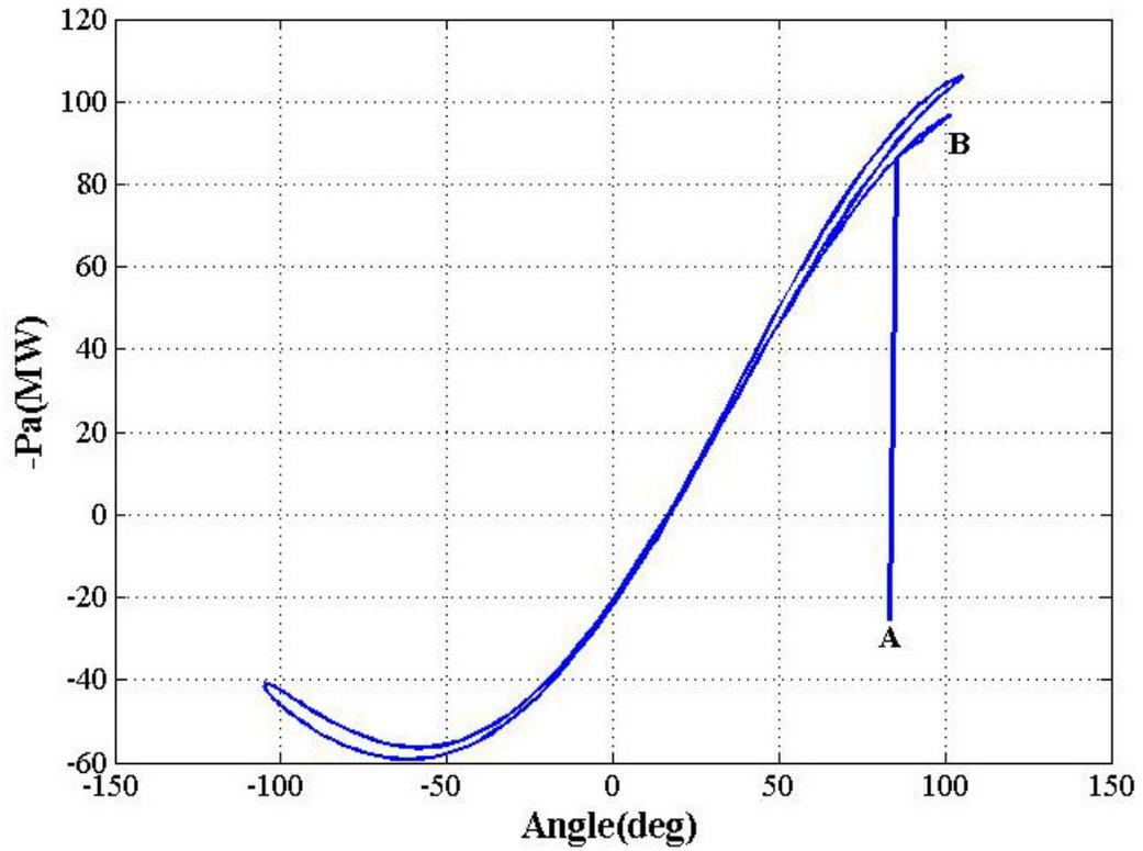
Figure 4.23 OMIB equivalent  $P$ - $\delta$  curve for case SIEQ.
