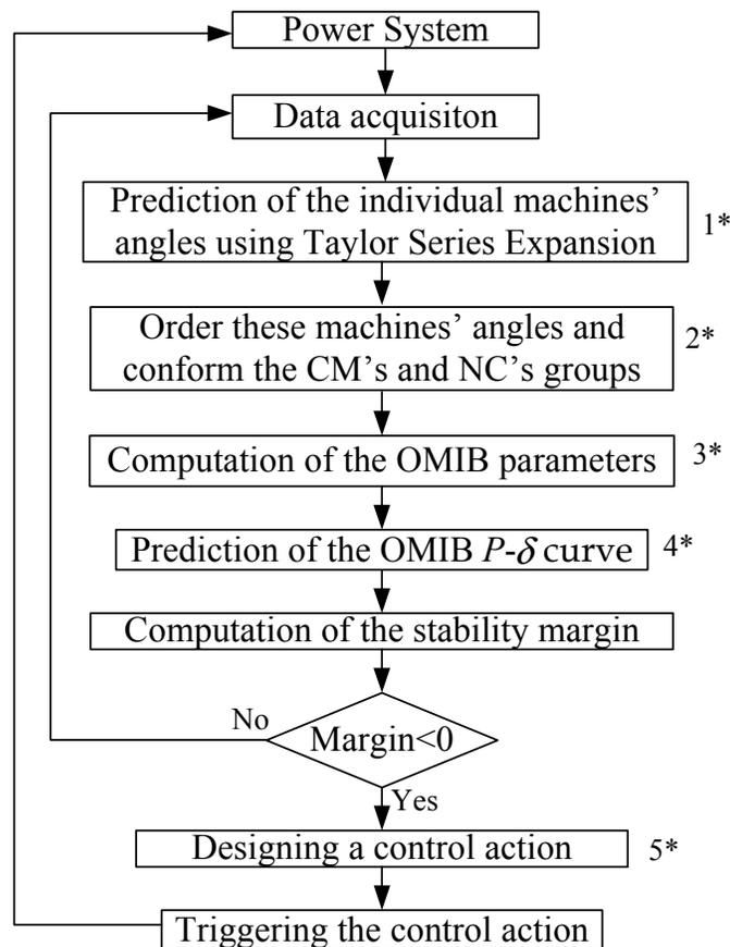
Figure 3.11 General flow diagram of the E-SIME method computational program.
