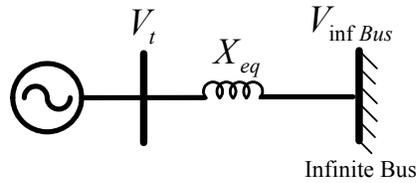
Figure 2.6 Basic one-machine infinite bus system.
