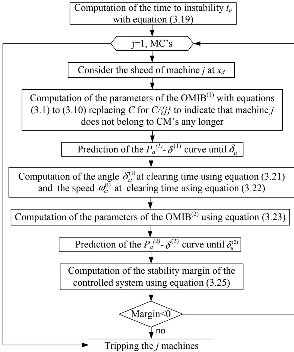
Figure 3.15 Flow diagram of the emergency control action design step.
