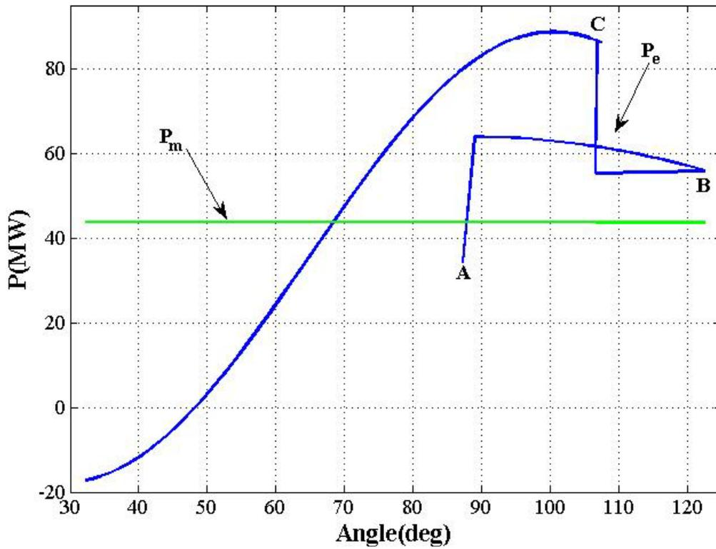
Figure 4.5 OMIB equivalent mechanical and electrical powers for case 1A.
