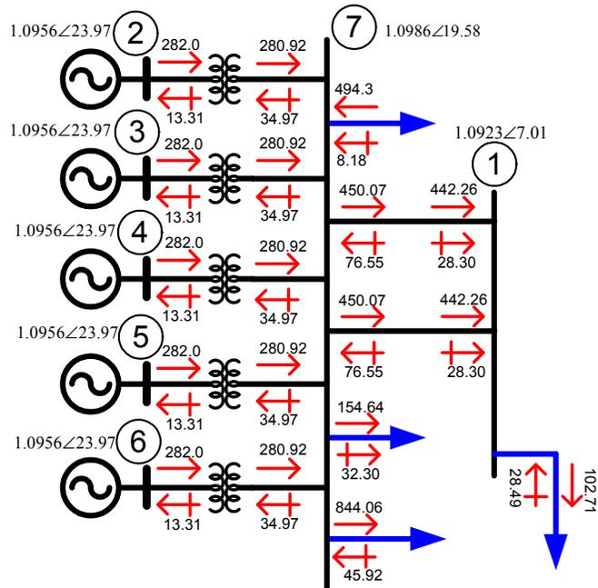
Figure A.1 One-line diagram of equivalent MMT test system
