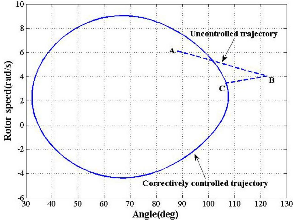
Figure 4.7 OMIB equivalent phase plane for case 1A: Stabilized system.
