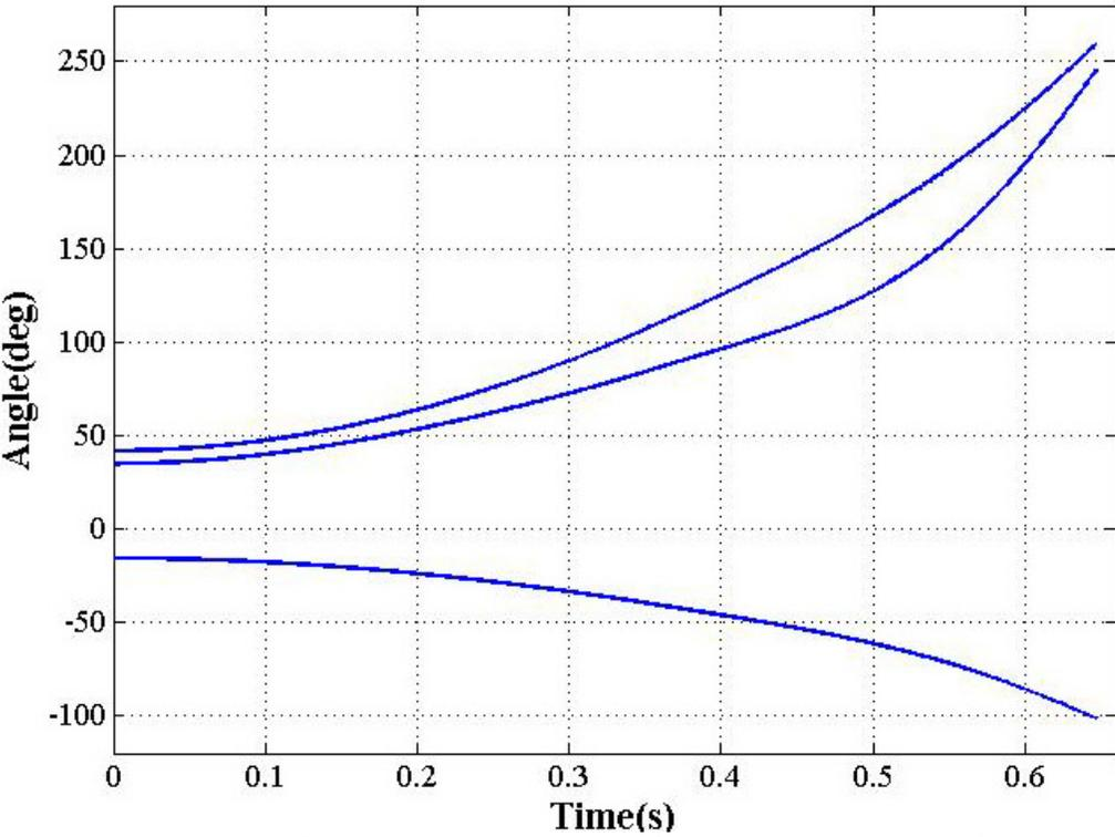
Figure 4.12  $\delta-t$  curve of the individual machines after the corrective action for case 3A.
