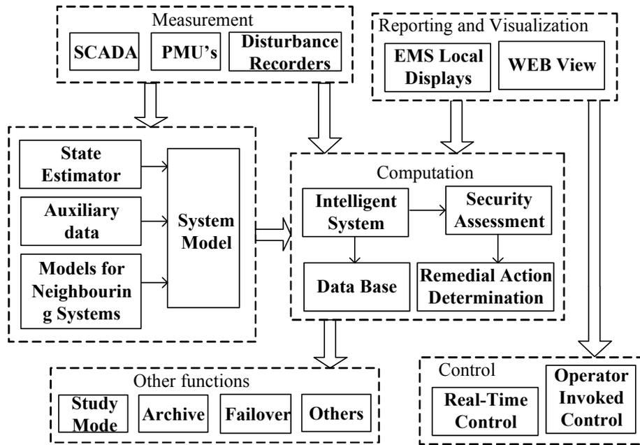
Figure 2.13 Components of an on-line dynamic security assessment system (Adapted from [CIGRE, 2007]).
