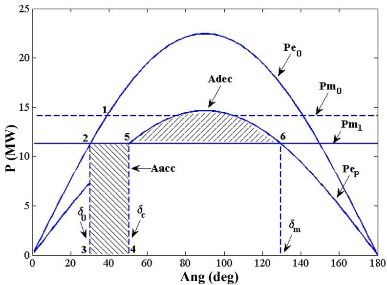
Figure 2.11 Stabilized case for the MMT power system using preventive control.
