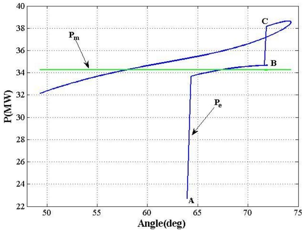
Figure 4.18 OMIB equivalent mechanical and electrical powers for case 1NE.
