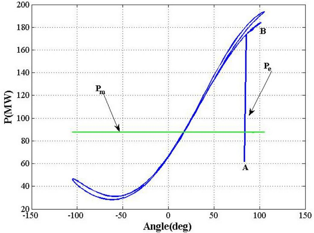
Figure 4.24 OMIB equivalent mechanical and electrical powers for case SIEQ.
