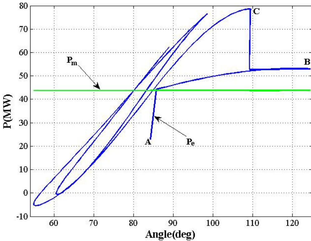
Figure 3.7 OMIB mechanical and electrical powers of the example case showing the action of E-SIME to stabilize the system. Points A, B, and C are included for a straightforward comparison with Fig. 3.5.
