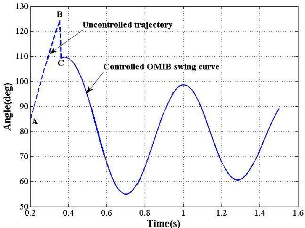
Figure 3.8 OMIB swing curve of the example case showing the action of E-SIME to stabilize the system. Points A, B, and C are included for a straightforward comparison with Fig. 3.5.
