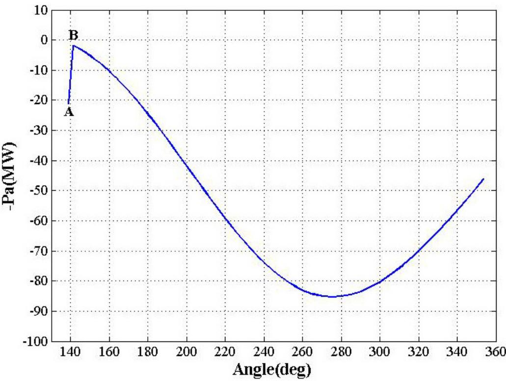
Figure 4.13  $P-\delta$  curve of the OMIB for the case 3A.
