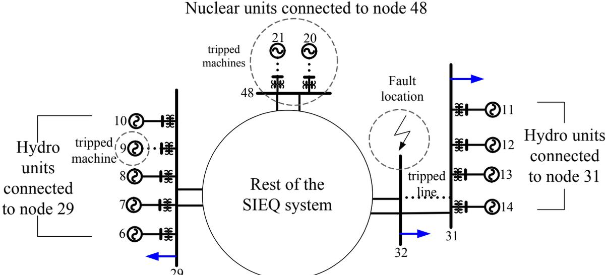
Figure 4.28 Application of the E-SIME method to the SIEQ test system.
