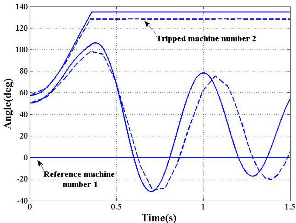
Figure B.2 Individual machines swing curves for the example case.
