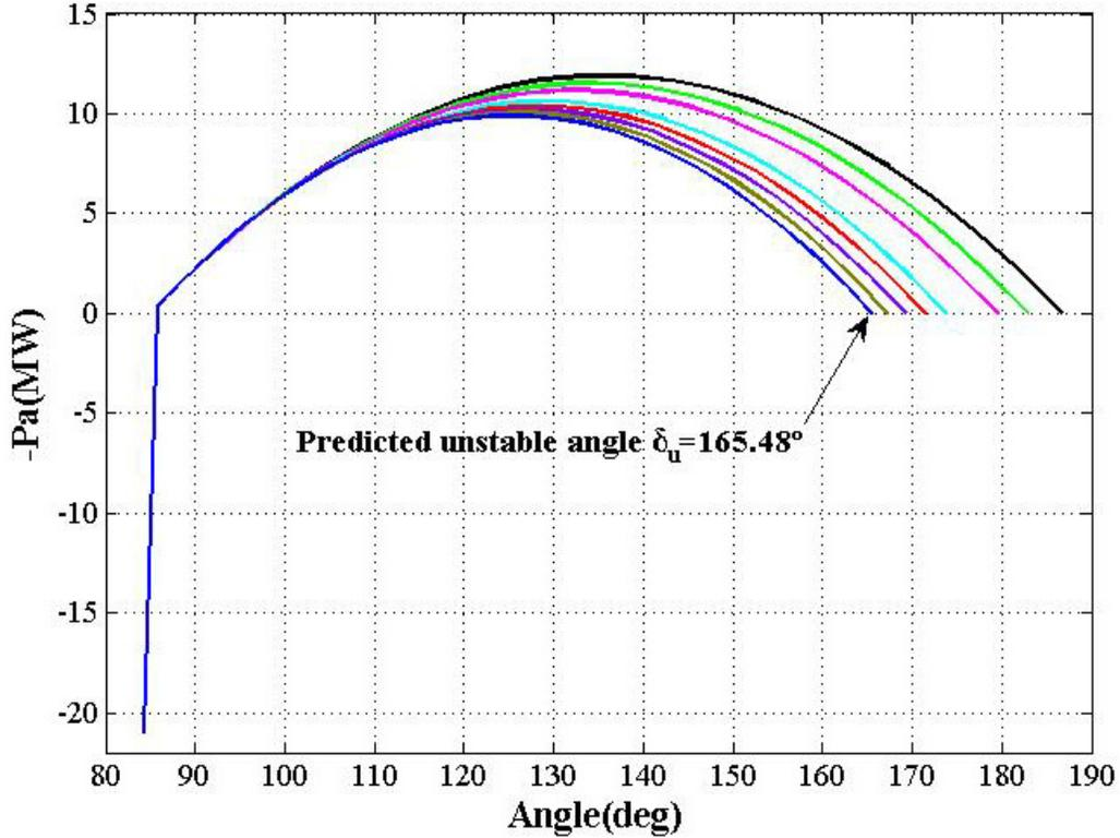
Figure 3.4 Prediction of the Pa- $\delta$  curve of the three-machine test system for the example case.
