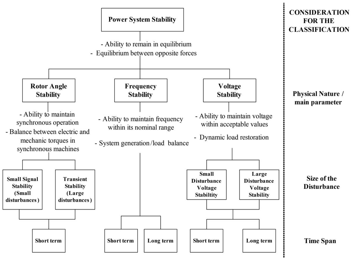
Figure 2.3 Power Systems Transient Stability Classification (Adapted from [IEEE, 2004]).
