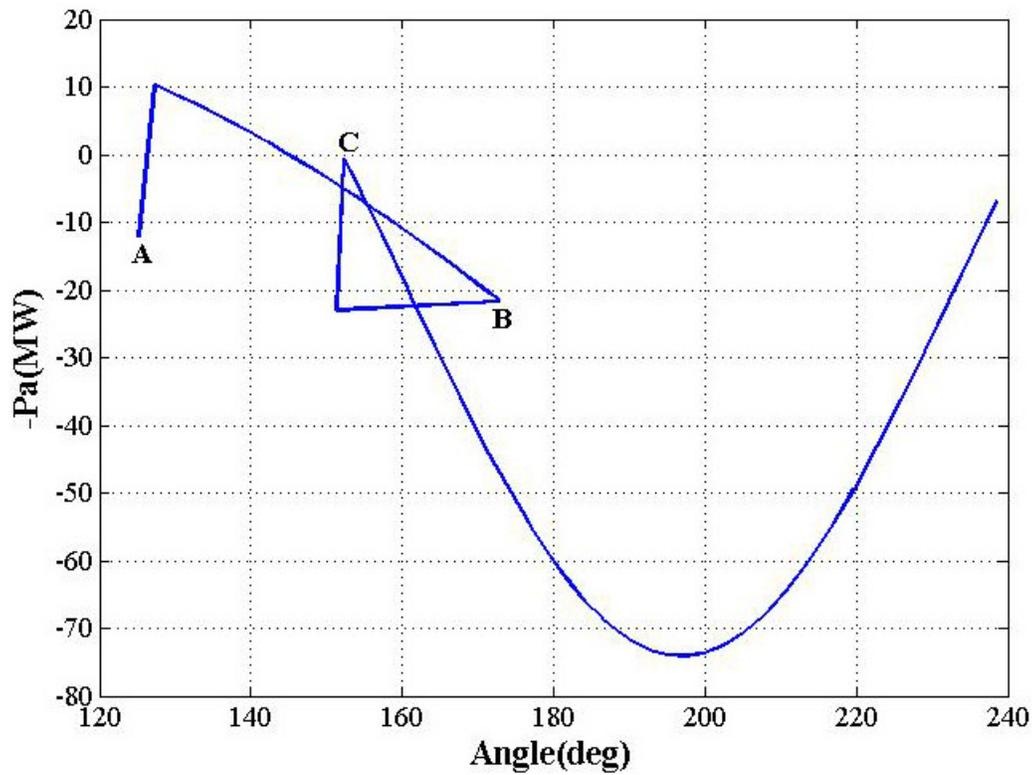
Figure 4.10 OMIB equivalent  $P-\delta$  curve for case 2A.
