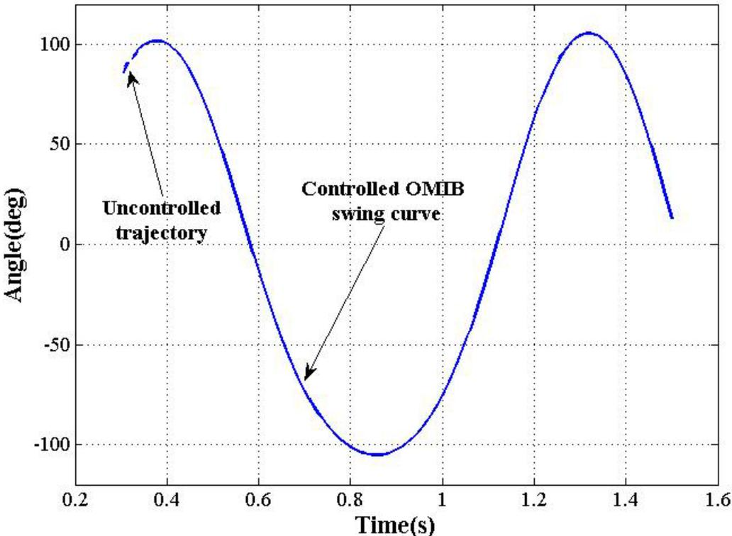
Figure 4.25 OMIB equivalent swing curve for case SIEQ: Stabilized system.
