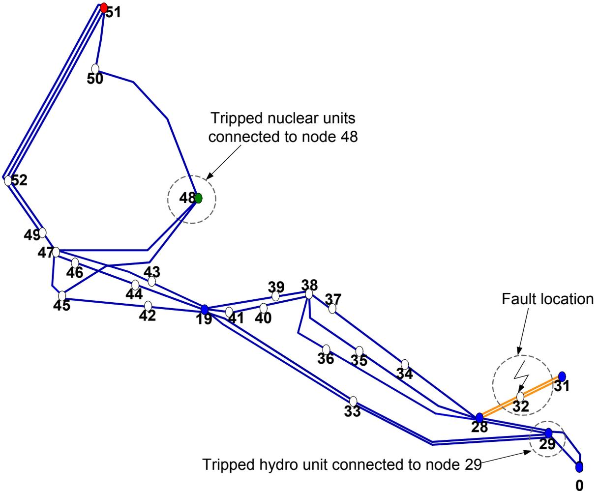
Figure 4.27 Application of the E-SIME method to the SIEQ test system.
