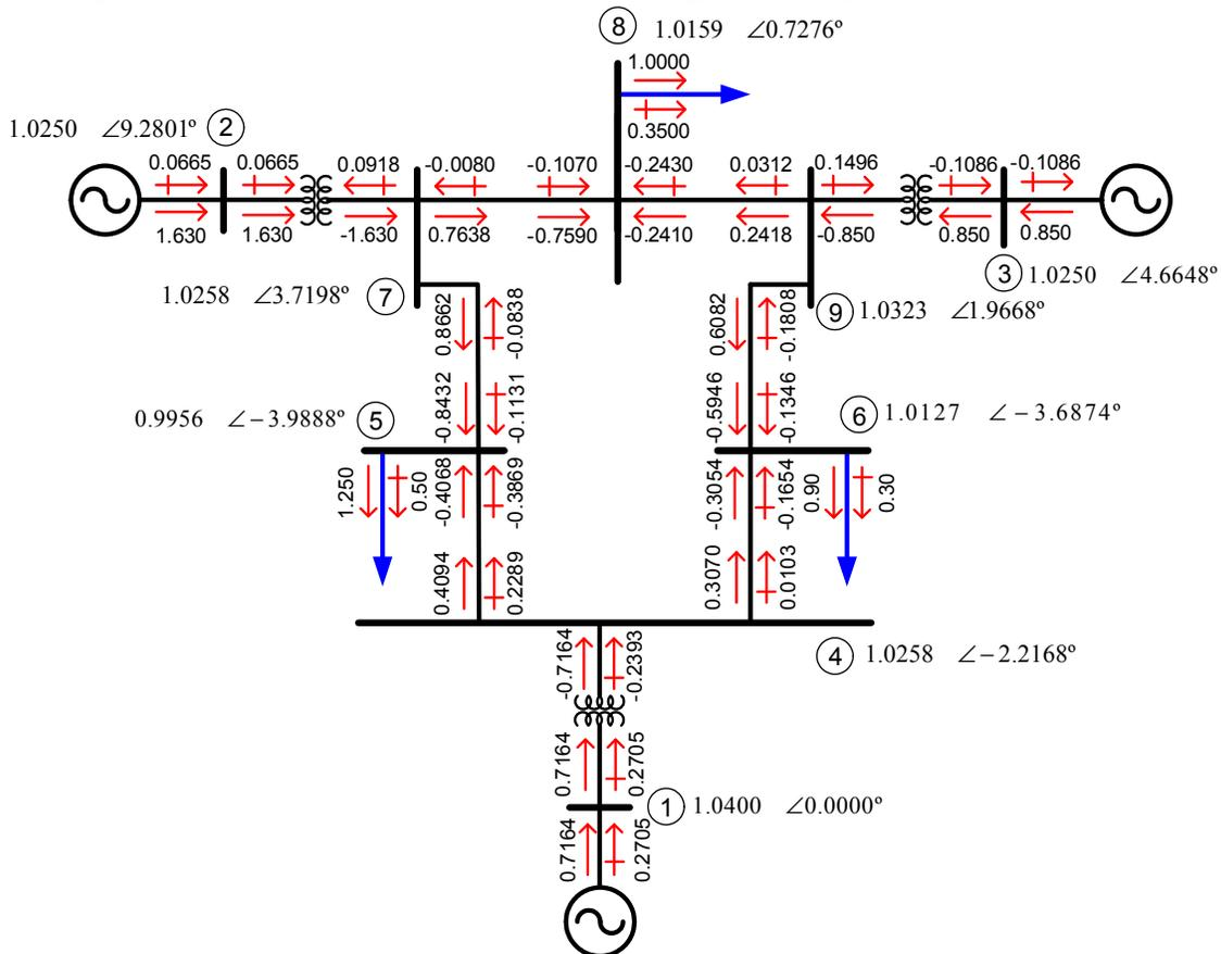
Figure A.2 One-line diagram of the three-machine test system (Adapted from [Anderson and Fouad, 1993]).
