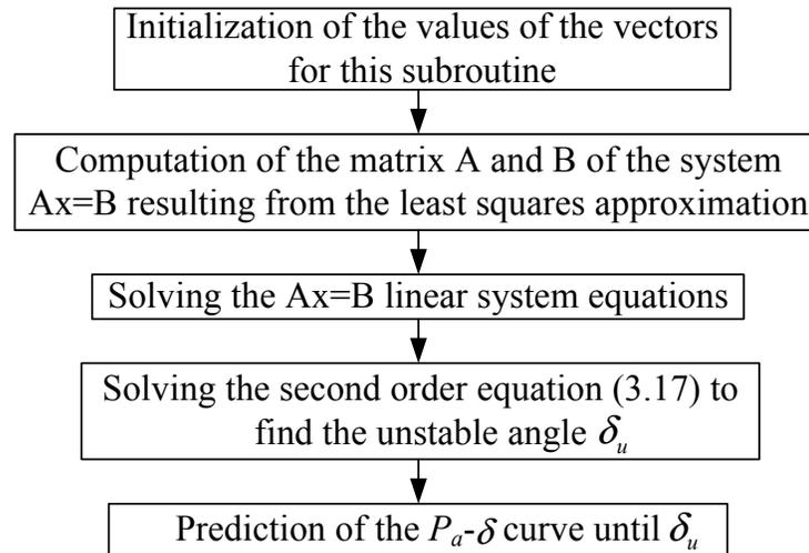
Figure 3.14 Flow diagram of the prediction of the  $P_a - \delta$  curve.
