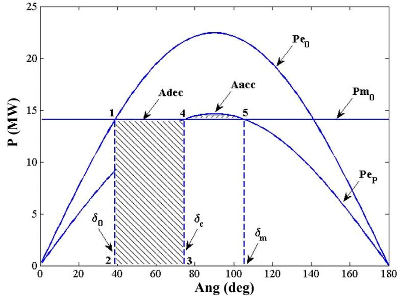
Figure 2.10 Unstable case for the MMT power system.
