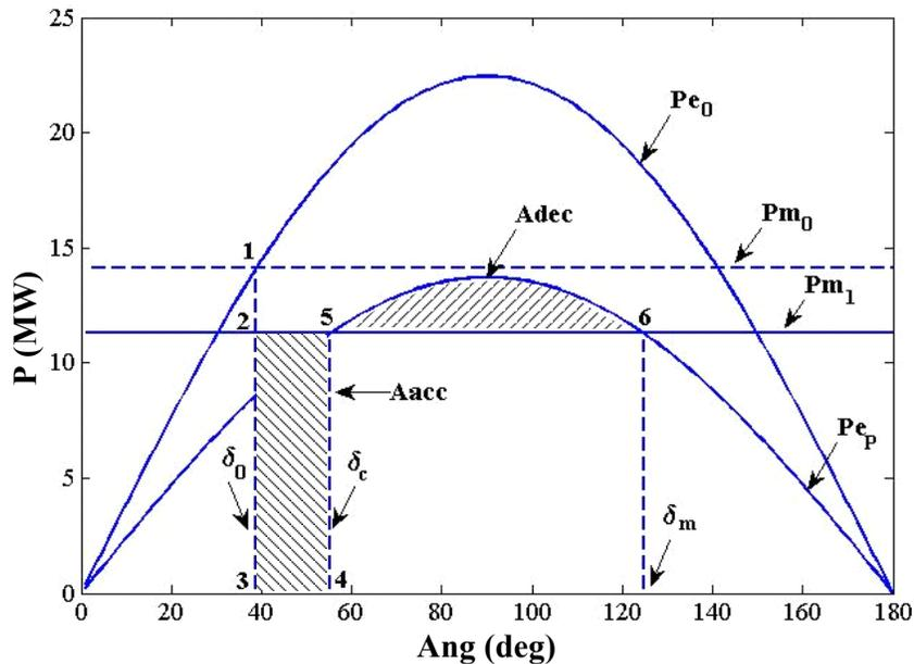
Figure 2.12 Stabilized case for the MMT power system using emergency control.
