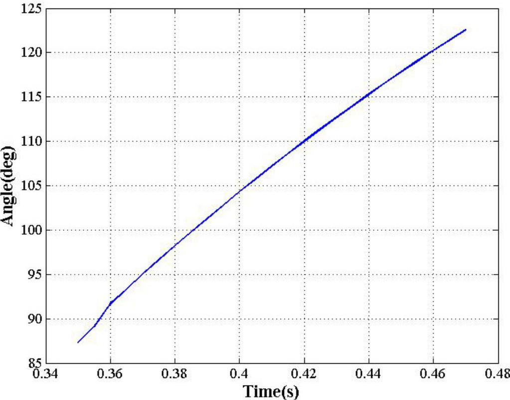
Figure 4.2 OMIB equivalent angle trajectory before the control action is applied for case 1A.
