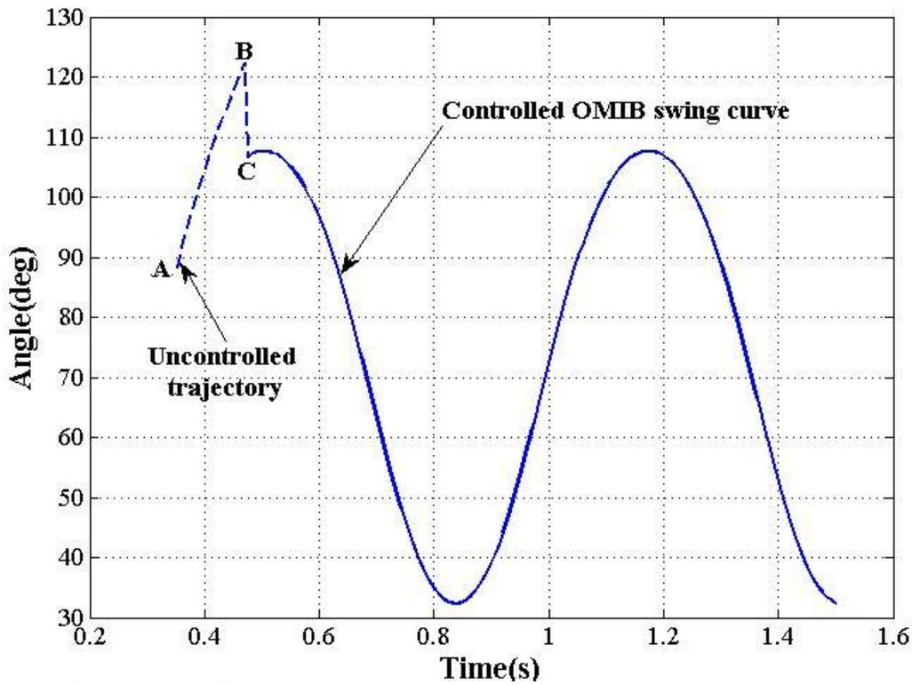
Figure 4.6 OMIB equivalent swing curve for the case 1A: Stabilized system.
