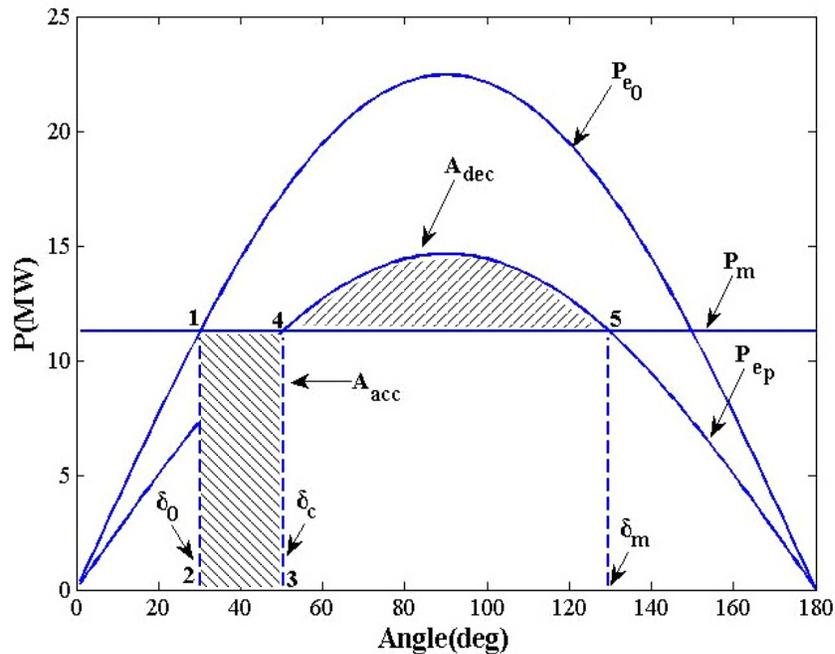
Figure 2.7 EAC of an infinite bus machine equivalent.
