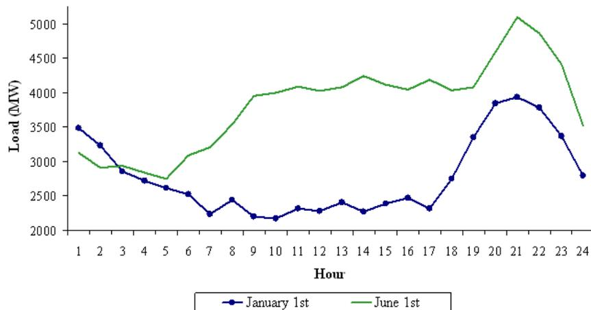
Figure 2.2 Measured values of the Mexican National interconnected power system during two different days in two different seasons in 1995 (Adapted from [Ruiz-Vega, 2002a]).
