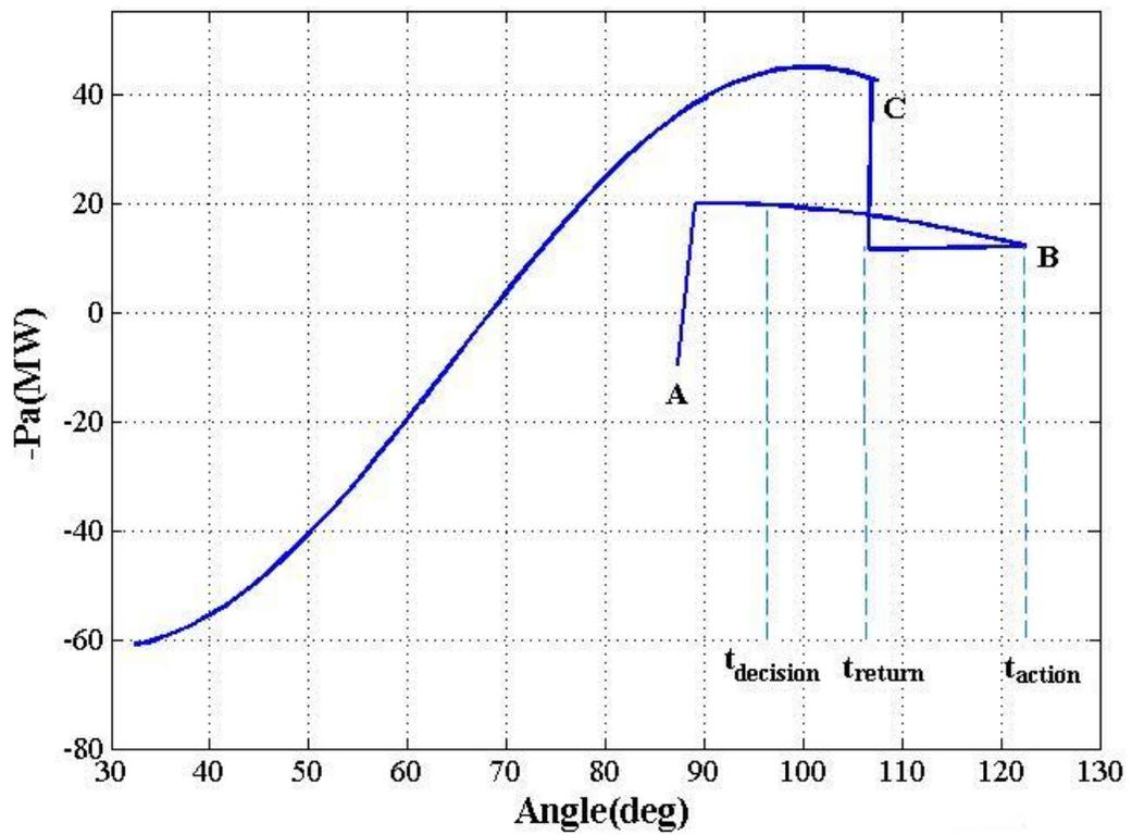
Figure 4.4 OMIB equivalent  $P-\delta$  curve for case 1A.
