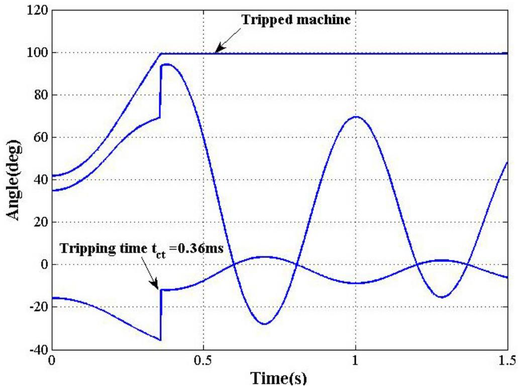
Figure 3.5 Swing curves of the individual machines of the example case showing the action of E-SIME to stabilize the system. After tripping machine 2 its angle value remains constant.
