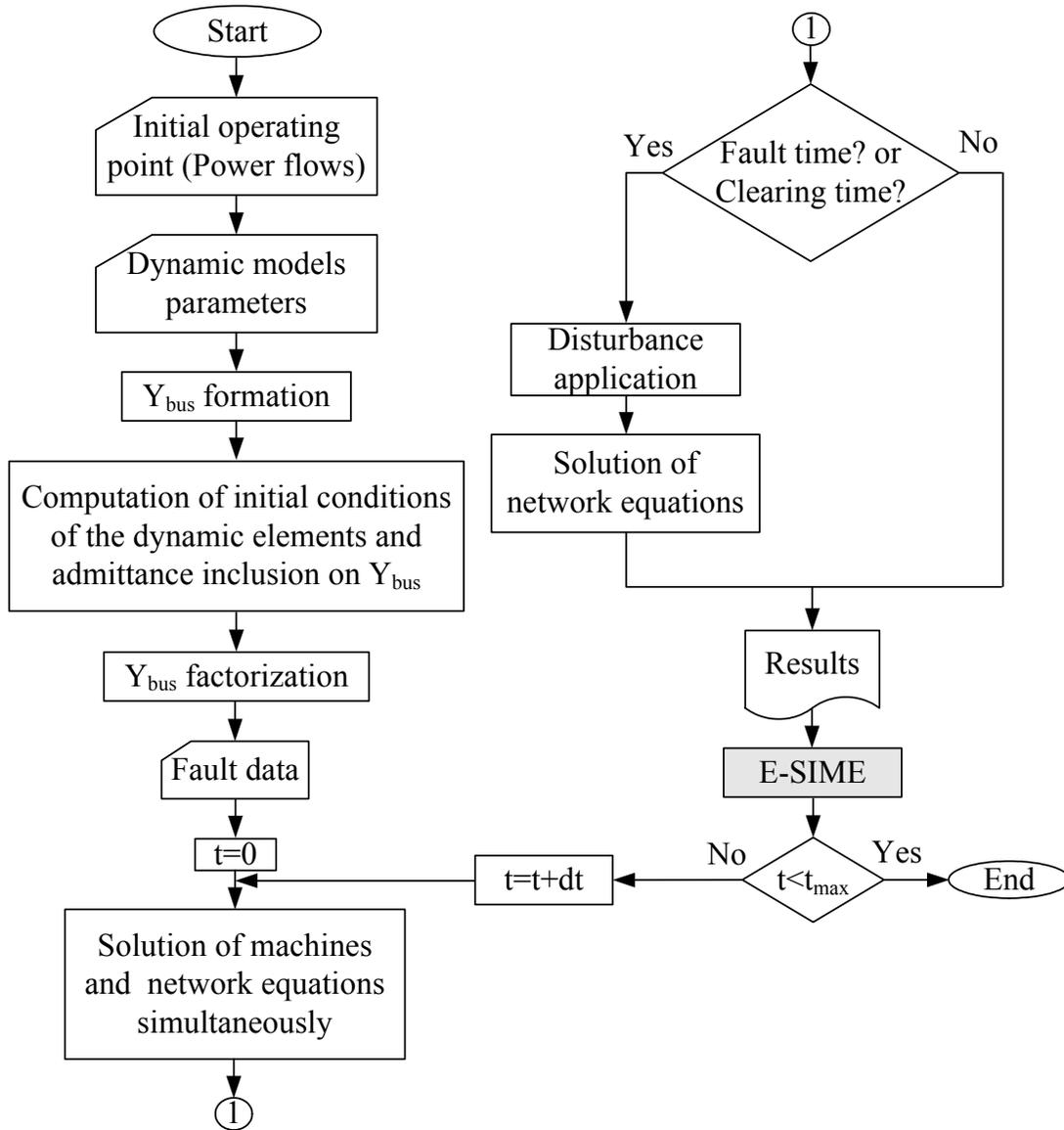
Figure 3.16 Flow diagram of the coupling of TRANSTAB and E-SIME programs.
