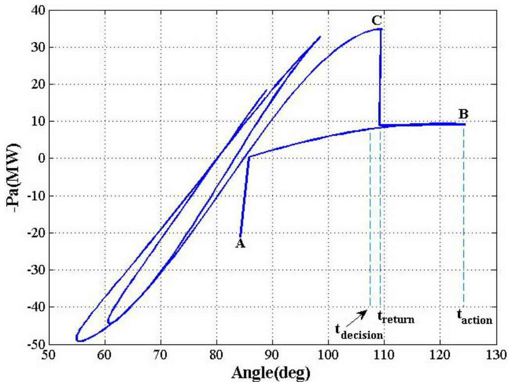
Figure 3.6  $P_a-\delta$  curve of the OMIB of the example case showing the action of E-SIME to stabilize the system. Time of the different assessment and control steps of E-SIME are indicated.
