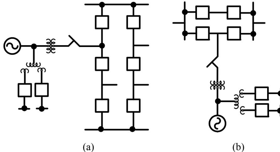
Figure 2.9 (a) Typical breaker-and-a-half station.
