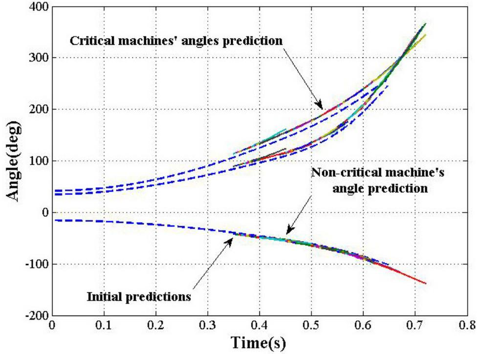
Figure 3.3 Taylor Series prediction of the three-machine test system for the example case.
