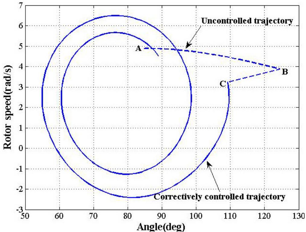
Figure 3.9 OMIB phase plane of the example case showing the action of E-SIME to stabilize the system. Points A, B, and C are included for a straightforward comparison with Fig. 3.5.
