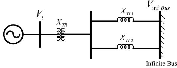
Figure 2.5 One-machine infinite bus system (Adapted from [Kundur, 1994]).
