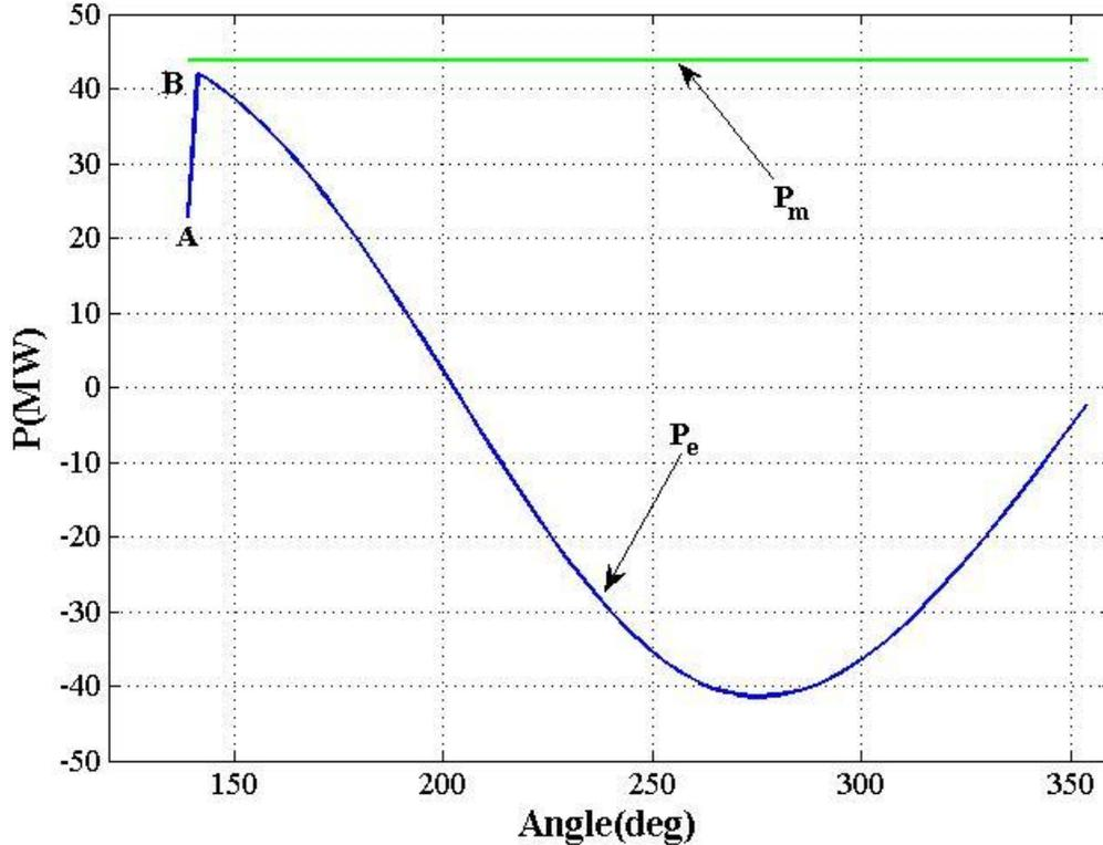
Figure 4.14 Mechanical and electrical powers of the OMIB for the case 3A.
