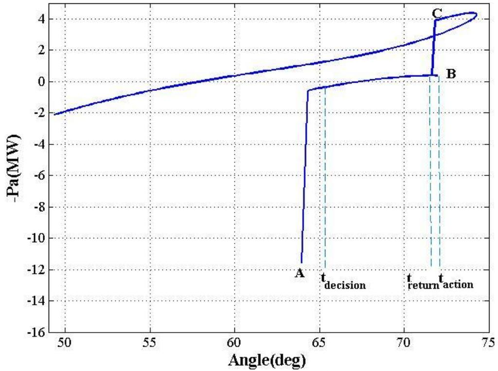
Figure 4.17 OMIB equivalent  $P-\delta$  curve for case 1NE.
