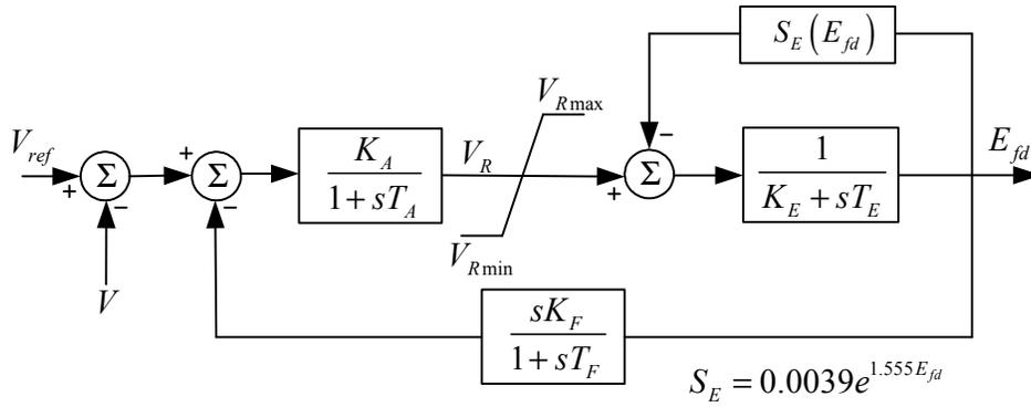
Figure A.3 Automatic Voltage Regulator type 1 model
